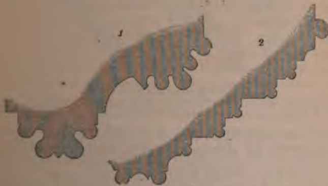
Sections of Pier-arches, St. Patrick's.
